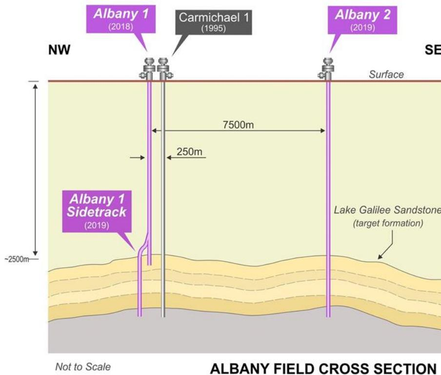
Figure 1: Cross Section of the Albany Field (courtesy of Comet Ridge)
